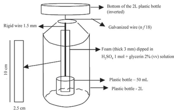
Figure 2. Scheme of the semi-open static ammonia collector (adopted from Araújo et al., 2009).
