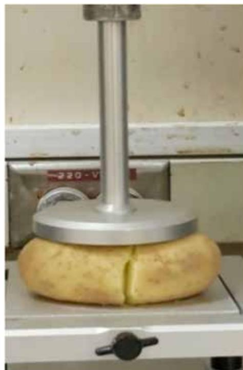
Figure 4. Force-deformation of food materials (ASAE, 2002).
