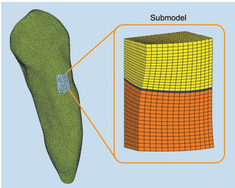
Fig. 2. Submodel of crown margin.
