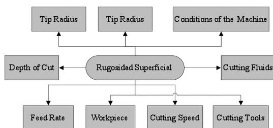
Figure 1. The major factors which affect the surface roughness.
