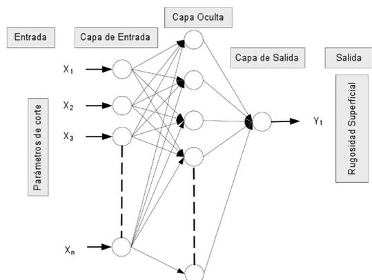
Figure 2. Structure of the multilayer perceptron network.
