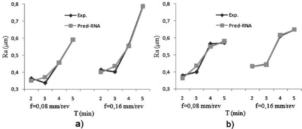
Figure 4. Measured values and estimated by artificial neural networks for  $v = 400 \text{ m min}^{-1}$ , a) was inserted GC1115 and, b) was inserted GC2015.
