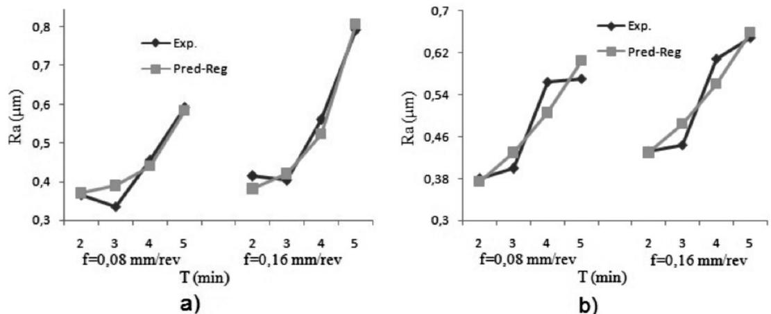
Figure 2a. Values measured and estimated by multiple regression for v = 400 m min<sup>-1</sup>, a) was inserted GC1115; and b) was inserted GC2015.
