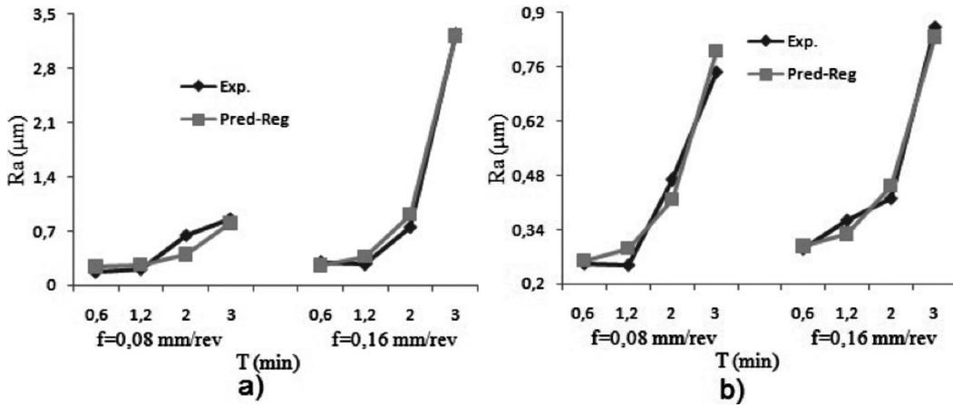
Figure 3. Measured values and estimated by multiple regression for  $v = 450 \text{ m min}^{-1}$ , a) was inserted GC1115; b) was inserted GC2015.
