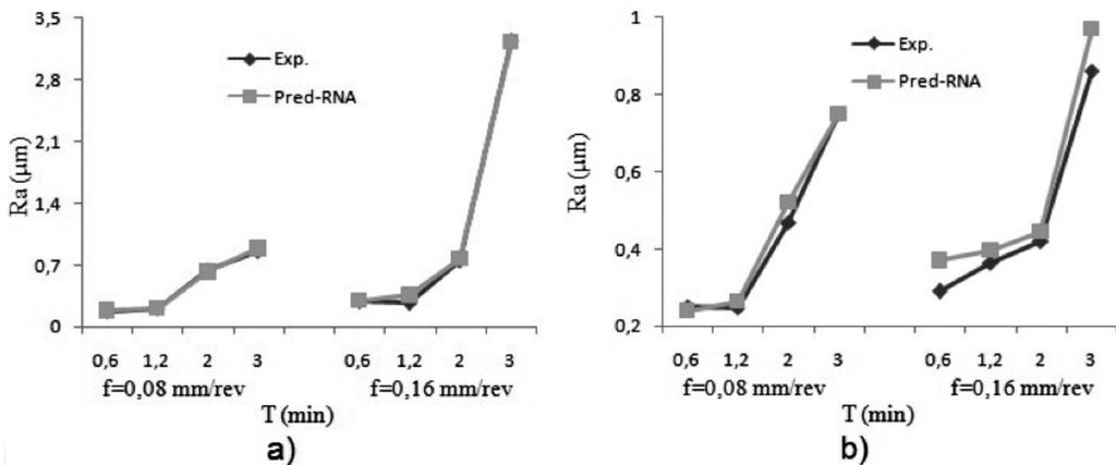
Figure 5. Measured values and estimated by artificial neural networks for  $v = 450 \text{ m min}^{-1}$ , a) was insert GC1115 y b) was insert GC2015.
