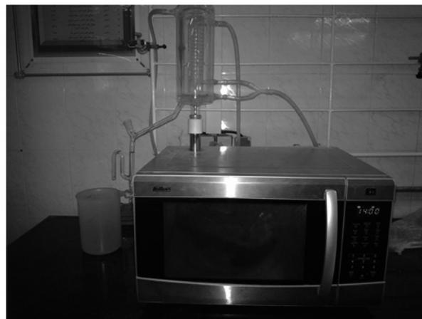
Fig. 1 – Microwave-assisted hydro-distillation apparatus used in this study.
