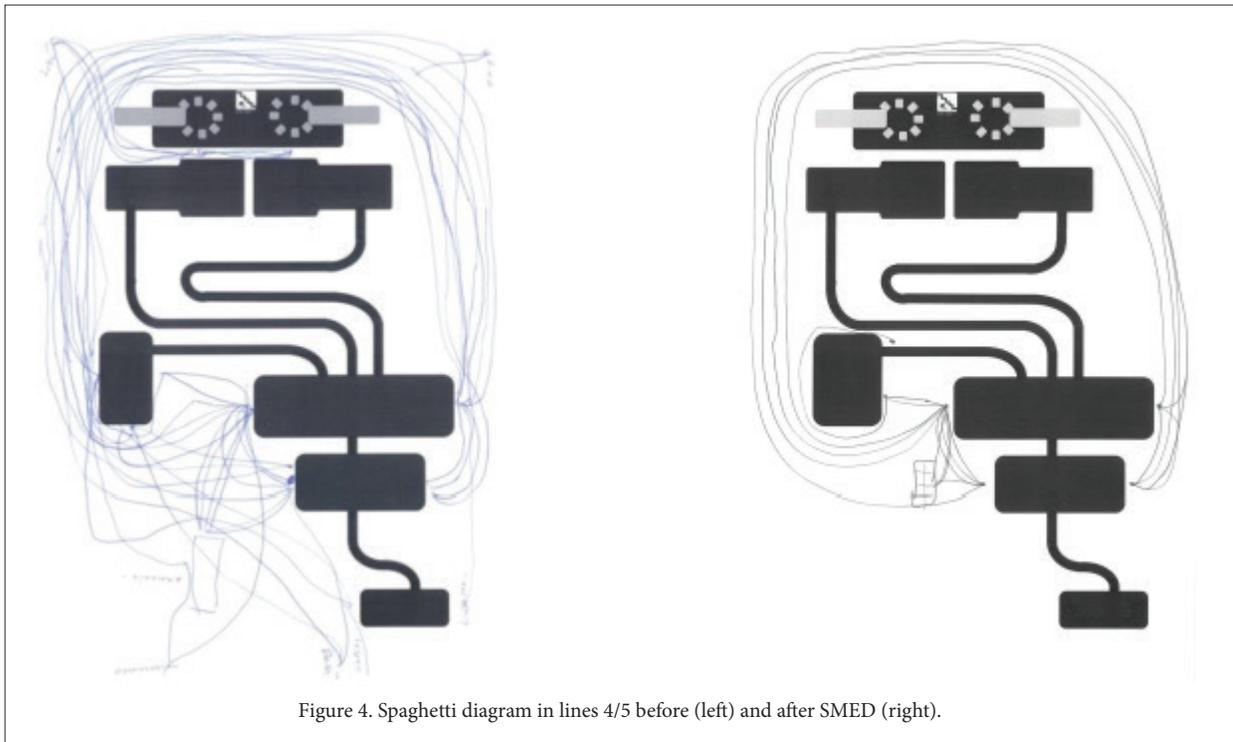
Figure 4. Spaghetti diagram in lines 4/5 before (left) and after SMED (right).
