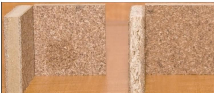
**Figure 2.** Photos of panels, from left to right: mixed panel with outer bark of white birch in the face and wood fibres in the core; mixed panel with outer bark of white birch in the face and wood particles in the core
