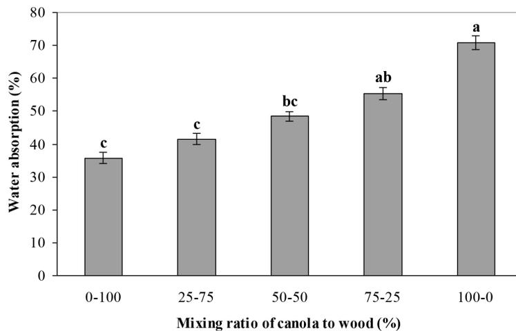
**Figure 4.** Water absorption of experimental panels for 24 h immersion in water (values are mean ± standard deviation).
