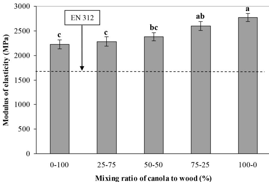
Figure 2. Modulus of elasticity of experimental panels (values are mean ± standard deviation).
