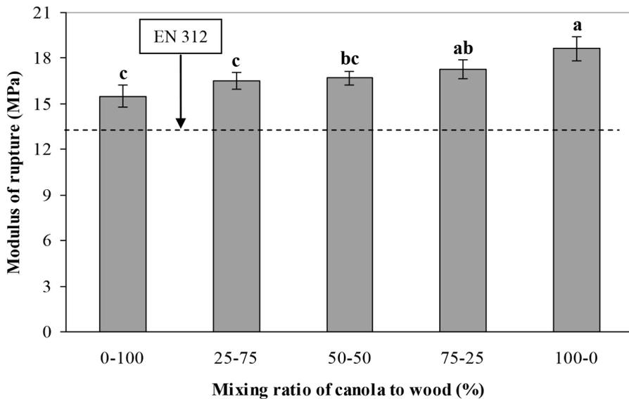
Figure 1. Modulus of rupture of experimental panels (values are mean ± standard deviation).
