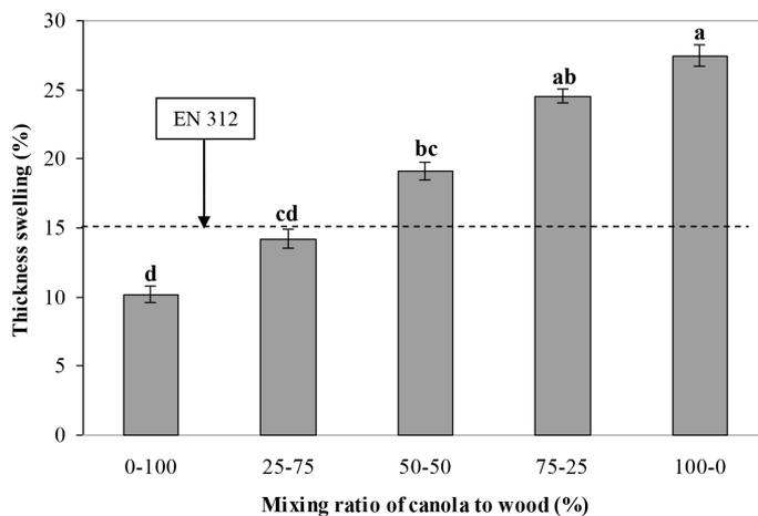
**Figure 5.** Thickness swelling of experimental panels for 24 h immersion in water (values are mean ± standard deviation).
