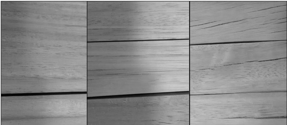
**Figure 1.** Surface appearance of MW treated eucalyptus wood. Left: 290 MJm<sup>-3</sup>(D1); Center: 360 MJm<sup>-3</sup>(D2); Right: 430 MJm<sup>-3</sup>(D3).
