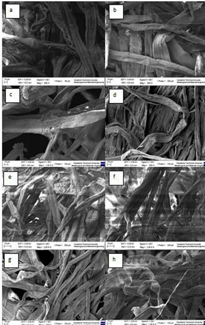
**Figure 1.** SEM photographs of the enzyme eucalypts and pine kraft pulp: (a) control of pine kraft pulp; (b) XyzGeo71 treatment of pine kraft pulp; (c) LipRHA1 treatment of pine kraft pulp; (d) consecutive XyzGeo71 and LipRHA1 treatment of pine kraft pulp; (e) control of eucalypts kraft pulp; (f) XyzGeo71 treatment of eucalypts kraft pulp; (g) LipRHA1 treatment of eucalypts kraft pulp; (h) consecutive XyzGeo71 and LipRHA1 treatment of eucalypts kraft pulp
